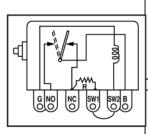
518APH Allows for SWICHGAGE® and/or N.C. contacts to be wired "Closed Loop" (in series). Any contact open or SWICHGAGE® contact close in the circuit shunt trips the 518APH. Specify 12 or 24 VDC. Contacts 10 amps 24V. 14 amp fuse.
