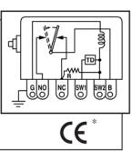
**760A/760AF/761APH** Use for distributor ignition or diesel. Time delay lockout of SWICH-GAGE® contacts on start-up only; customer wired for delayed or immediate trip on shutdown. Breaks and makes circuits when tripped. 760A resets automatically when the shutdown signal is removed or power is removed. 761APH has manual reset. 760AF is 760A with inline fuse. Must specify 12 or 24 VDC, and length of time delay. Ontional time delays: 15, 3
